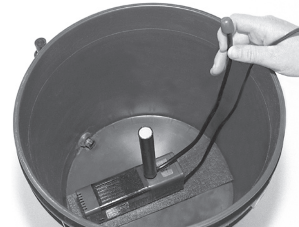
Place pump assembly inside reservoir. The pump output should point straight up so that the spray hits the spray-diffuser under the center of the reservoir cover.
